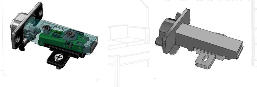
There is differents ways to simplify a geometry (Part/Assembly Simplified representation, tolerancy...)
